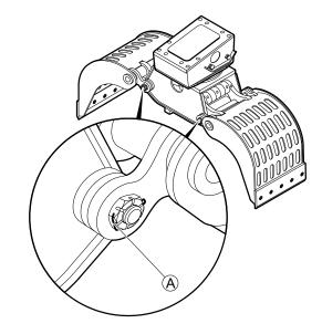
Replace damaged castle nuts and splint pins.
