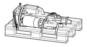
Move the fork of the forklift truck under the pallet so that the hydraulic attachment cannot tip over.
