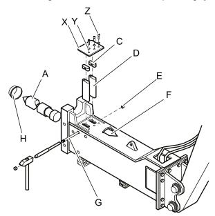
Wiper installed (only hydraulic breakers with DustProtector):
