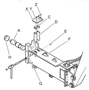
Wiper installed (only hydraulic breakers with DustProtector):
