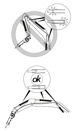
These end positions have damping facilities; the hydraulic cylinder may be damaged by prolonged use while in its end positions.
