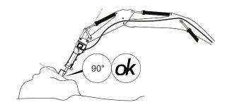
If you do not do this, the hydraulic breaker will wear faster and damage will occur after a while.
