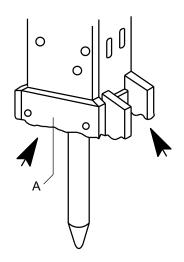
If the wear rails have worn severely, this may cause damage to the basic body of the breaker box.
