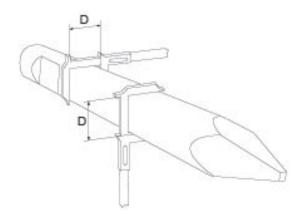
Replace the working tool if the shaft has worn to the minimum diameter D<sub>min</sub> stated below.
