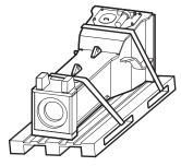
Move the fork of the forklift truck under the pallet so that the hydraulic attachment cannot tip over.
