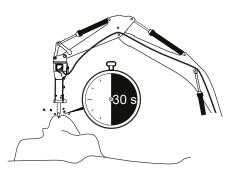
If the material fails to break, apply the tool to a new location.
