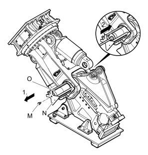
Disassemble the bolt cage (N).
