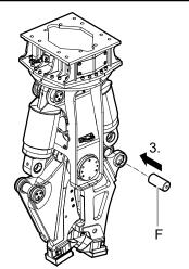
Place the hydraulic demolition cutter with the broad back of the cutter jaw (double) on the assembly rack so that the pin lies in the semi-shell of the assembly rack.
