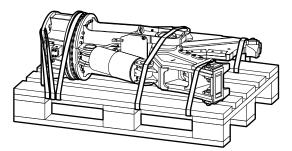
Move the fork of the forklift truck under the pallet so that the hydraulic attachment cannot tip over.
