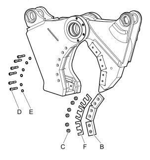
Re-check the blade clearance (see chapter Correcting the blade clearance). Repeat this procedure until the blade clearance is less than 0.2 mm (0.008 in.).
