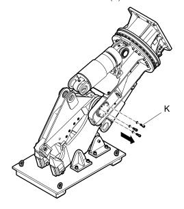
The bolt cage has two Allen screws.
