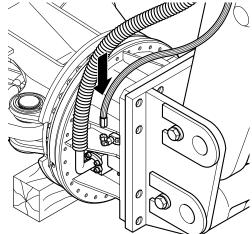
■ Connect both hoses for the function »Turn« at the boom in a torsion-free manner.
