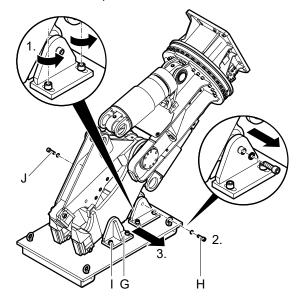
■ Lift the hydraulic demolition cutter.
