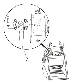
17. Fit the pressure line (C) to the bucket crusher's connections and the shut-off valve on the carrier in a torsion-free manner.
