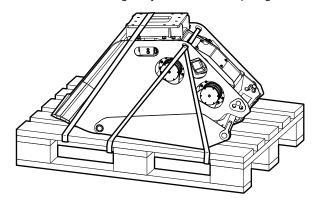
Move the fork of the forklift truck under the pallet so that the hydraulic attachment cannot tip over.
