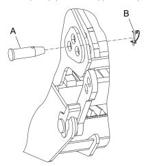
Remove the upper bolts (A), using a hammer if necessary.
