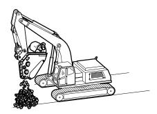
Once you have completely crushed the material deposited in the bucket crusher, repeat the operation of filling and crushing.
