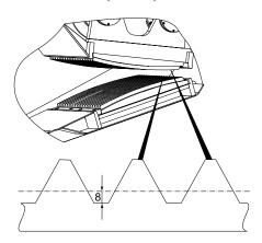
Change the jaws when the rails are worn on both ends to less than 8 mm (0.03 in.).
