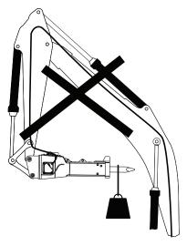
Never use the hydraulic breaker as a sledge hammer to demolish material.
