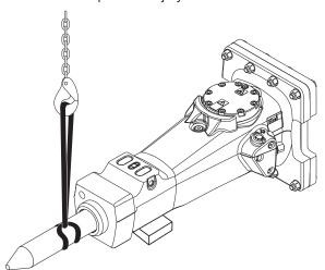
3. Remove and check the lock buffer. Change worn or damaged parts.
