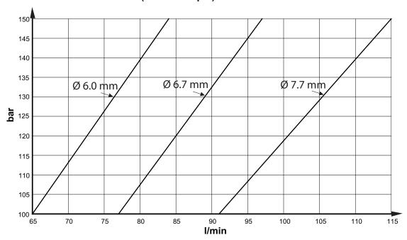
SB 552 Tunnel is delivered with restrictor Ø9.1 for 110 bar (1595 psi) operation. As an option, restrictor Ø7.7 for operation at higher pressure, is available.
