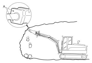
Use a permanent water flushing and air supply as standard to minimize wear and enable dust binding during operation. See "Hoses and connections" for information about connecting utilities.
