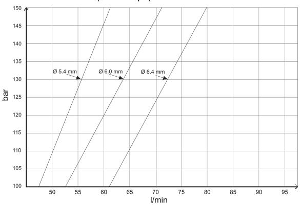
SB 302 Tunnel is delivered with restrictor Ø6.7 for 110 bar (1595 psi) operation. As an option, restrictor Ø6.4 for operation at higher pressure, is available.
