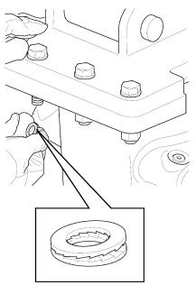
Tighten the nuts, see the tightening torque in the table below
