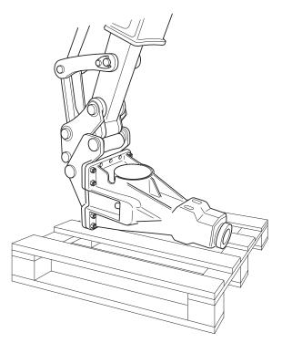
The pressure inlet on the hydraulic breaker is on the left side when you are facing the accumulator. If the pressure hose is on the other side of the boom you can cross the hoses or turn the hydraulic breaker.
