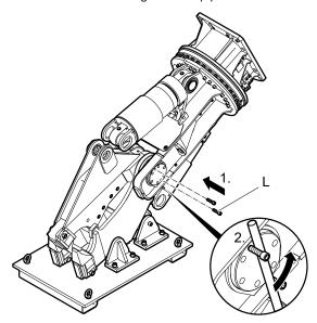
Remove the hexagon head screw (M) located in the middle of the main bearing pin.
