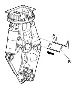
The piston rod sheaths are now prevented from slipping out.
