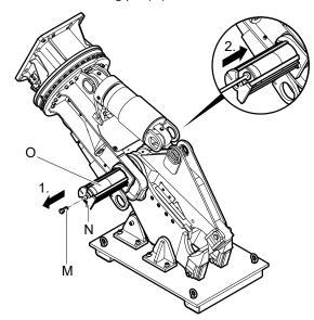
■ Disassemble the bolt cage (N).
