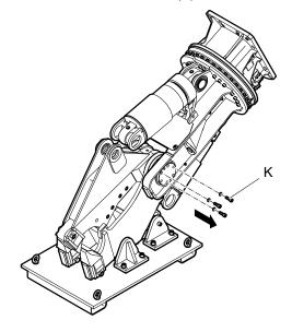
The bolt cage has two Allen screws.
