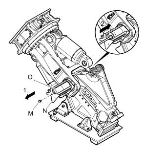
■ Disassemble the bolt cage (N).
