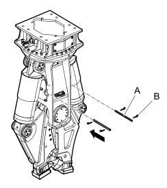
The piston rod sheaths are now prevented from slipping out.
