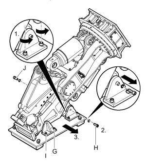
■ Lift the hydraulic demolition cutter.
