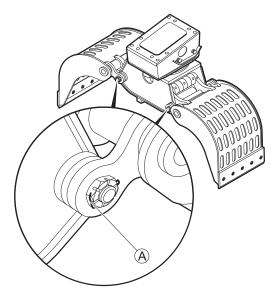
Replace damaged castle nuts and splint pins.
