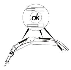
These end positions have damping facilities; the hydraulic cylinder may be damaged by prolonged use while in its end positions.
