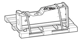
Move the fork of the forklift truck under the pallet so that the hydraulic attachment cannot tip over.
