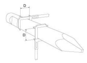
Replace the working tool if the shaft has worn to the minimum diameter D<sub>min</sub> stated below.
