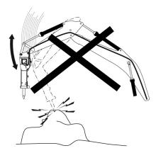
■ Never use the hydraulic breaker to move debris.
