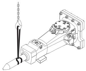
Remove and check the lock buffer. Change worn or damaged parts.
