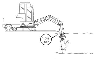
NOTICE Damage to the hydraulic breaker
