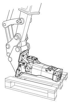
The pressure inlet on the hydraulic breaker is on the left side when you are facing the accumulator. If the pressure hose is on the other side of the boom you can cross the hoses or turn the hydraulic breaker.
