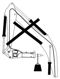
Never use the hydraulic breaker as a sledge hammer to demolish material.
