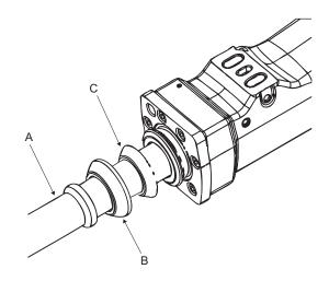
For Tunnel versions, dismount the working tool (A), front shield (B) and dust cover (C). Use a lifting strap to reduce the risk of personal injury.
