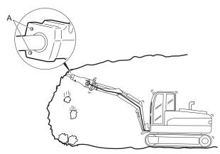
Use a permanent water flushing and air supply as standard to minimize wear and enable dust binding during operation. See "Hoses and connections" for information about connecting utilities.
