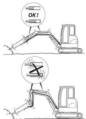
Avoid idling strokes; it causes wear on both working tool and tool retainers.
