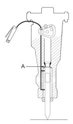
2. Lubricate the working tool's shank plentifully during all upward operations. The bushing and the working tool must be lubricated so frequently that dirt cannot penetrate into the hydraulic breaker.
