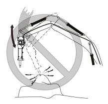
This will damage the hydraulic breaker, the working tool and the carrier.
