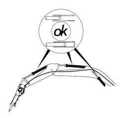
These end positions have damping facilities; the hydraulic cylinder may be damaged by prolonged use while in its end positions.
