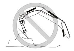
Slightly swing the hydraulic breaker to and fro when carrying out the hammer impacts, but never swing it through more than approx. 5°.
