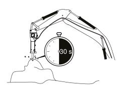
If the material fails to break, apply the tool to a new location.
