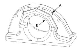
• the material is worn up to the checkpoints (A, B).
