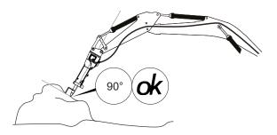
If you do not do this, the hydraulic breaker will wear faster and damage will occur after a while.
