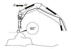
This swing action enables any dust under the tip or the cutter of the working tool to escape. Otherwise a layer of dust is created which would prevent the full percussion energy being transferred to the material to be broken. The tip of the working tool then becomes hot and loses its hardness. Larger swing angles would lead to bending loads and damage to the working tool and the hydraulic breaker.
