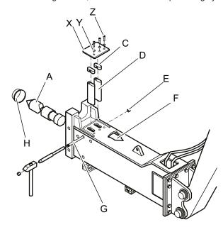
Wiper installed (only hydraulic breakers with DustProtector):
