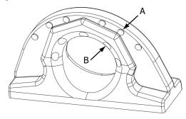
• the material is worn up to the checkpoints (A, B).
