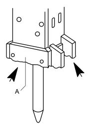
If the wear rails have worn severely, this may cause damage to the basic body of the breaker box.
