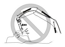
This might cause the working tool to break. Listen to the sound of the hydraulic breaker – it changes when stresses occur between the working tool and the wear bush.
