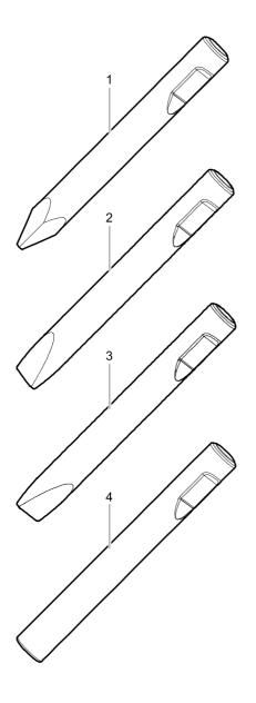
Ø=200 mm, L=815 mm, Lt=1650 mm, Wt=349.0 kg Ø=7.87 inch, L=32 inch, LT=64.96 inch, Wt=769.4 lb
