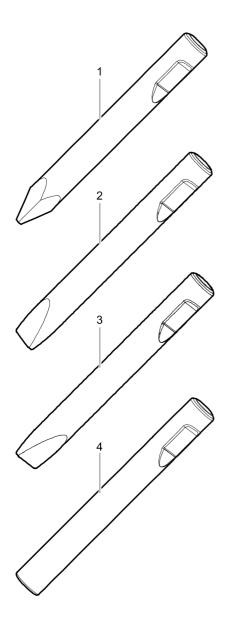
Ø=140 mm, L=670 mm, LT=1150 mm, Wt=120.7 kg Ø=5.51 inch, L=26 inch, LT=45.28 inch, Wt=266.1 lb
