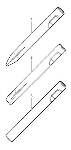
Ø=110 mm, L= 630 mm, LT=1100 mm, Wt=73.0 kg Ø=4.33 inch, L=25 inch, LT=43.31 inch, Wt=160.9 lb
