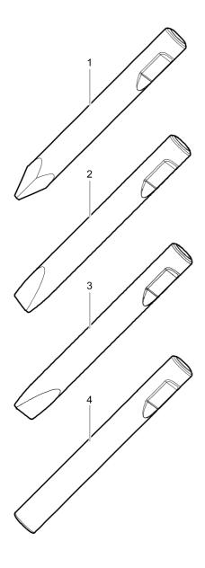
Ø=100 mm, L=510 mm, LT=920 mm, Wt=51.0 kg Ø=3.94 inch, L=20 inch, LT=36.22 inch, Wt=112.4 lb
