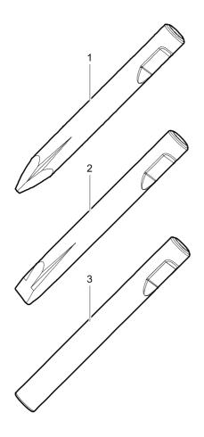
Ø=100 mm, L=590 mm, LT=1000 mm, Wt=55.0 kg Ø=3.94 inch, L=23 inch, LT=39.37 inch, Wt=121.3 lb
