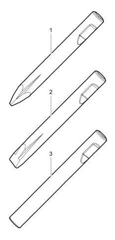
Ø=240 mm, L=880 mm, LT=1900 mm, Wt=570.0 kg Ø=9.45 inch, L=35 inch, LT=74.80 inch, Wt=1256.6 lb
