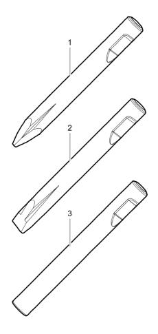
Ø=210 mm, L=935 mm, LT=1800 mm, Wt=417.0 kg Ø=8.27 inch, L=37 inch, LT=70.87 inch, Wt=919.3 lb
