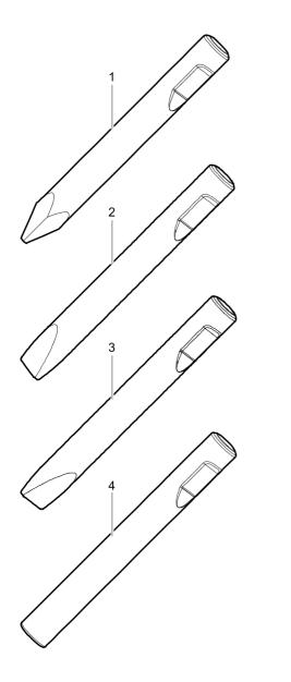
Ø=200 mm, L=760 mm, Lt=1650 mm, Wt=349.0 kg Ø=7.87 inch, L=30 inch, LT=64.96 inch, Wt=769.4 lb
