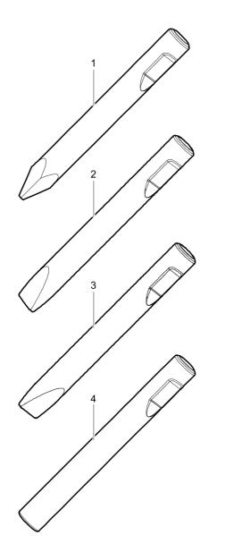
Ø=155 mm, L=640 mm, Lt=1310 mm, Wt=171.0 kg Ø=6.10 inch, L=25 inch, LT=51.57 inch, Wt=374.8 lb
