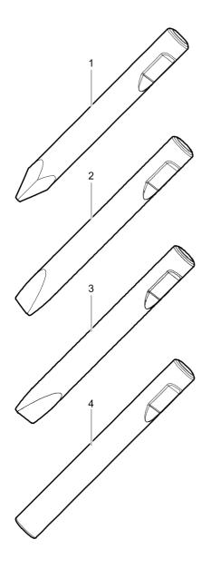
Ø=155 mm, L=640 mm, Lt=1310 mm, Wt=171.0 kg Ø=6.10 inch, L=25 inch, LT=51.57 inch, Wt=374.8 lb
