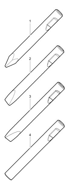
Ø=155 mm, L=600 mm, Lt=1310 mm, Wt=171.0 kg Ø=6.10 inch, L=24 inch, LT=51.57 inch, Wt=374.8 lb
