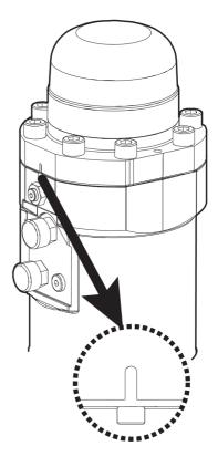
Install the back head onto cylinder housing where the marks meet each other.
