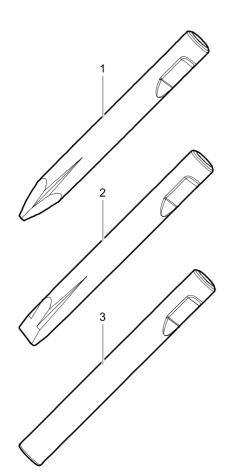
$\varnothing$ =180 mm, L=835 mm, L\_\_=1600 mm, Wt=277.0 kg  $\varnothing$ =7.09 inch, L=33 inch, L\_\_=62.99 inch, Wt=610.7 lb
