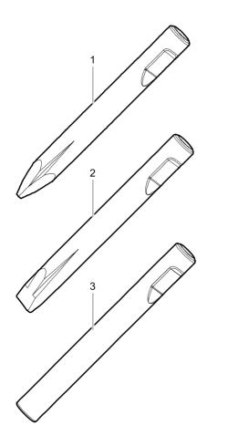
Ø=145 mm, L= 600 mm, LT=1230 mm, Wt=139.0 kg Ø=5.71 inch, L=24 inch, LT=48.43 inch, Wt=306.4 lb
