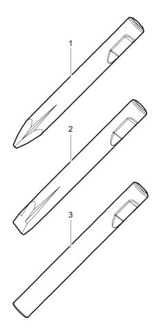
Ø=140 mm, L=670 mm, L $_{\rm T}$ =1200 mm, Wt=125.5 kg Ø=5.51 inch, L=26 inch, L $_{\rm T}$ =47.24, Wt=276.7 lb
