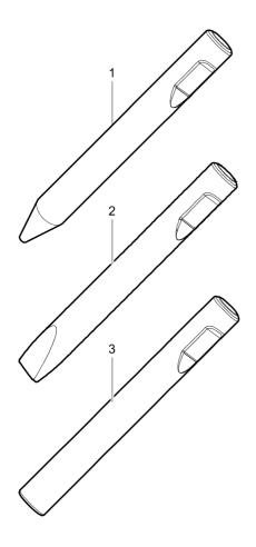
Ø=90 mm, L=460 mm, LT =835 mm, Wt=37.1 kg Ø=3.54 inch, L=18 inch, LT=32.87 inch, Wt=81.8 lb
