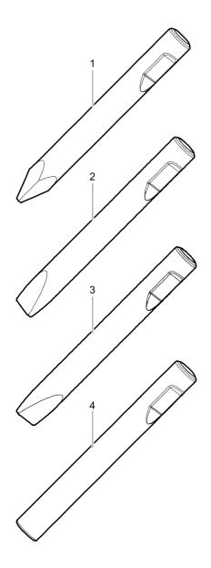
Ø=190 mm, L=730 mm, LT=1580 mm, Wt=306.0 kg Ø=7.48 inch, L=29 inch, LT=62.20 inch, Wt=674.6 lb
