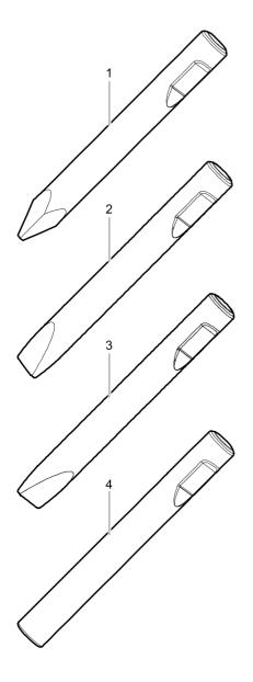
Ø=180 mm, L= 705 mm, LT=1530 mm, Wt=266.0 kg Ø=7.09 inch, L=28 inch, LT=60.24 inch, Wt=586.4 lb
