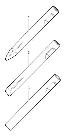
Ø=170 mm, L= 765 mm, LT=1500 mm, Wt=231.5 kg Ø=6.69 inch, L=30 inch, LT=59.06 inch, Wt=510.4 lb
