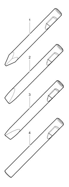
Ø=165 mm, L=675 mm, LT=1380 mm, Wt=198.1 kg Ø=6.50 inch, L=27 inch, LT=54.33 inch, Wt=436.7 lb
