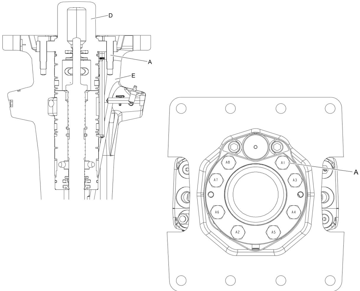
1. Press the back head (D) down on the hammer body(E).
